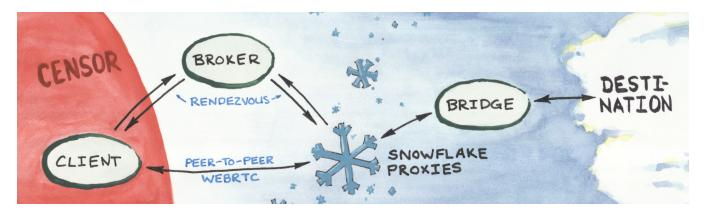
Figure 1: Architecture of Snowflake. The client contacts the broker through a special channel with high blocking resistance. The broker assigns the client a compatible proxy from among those currently polling. The client and proxy connect to one another using WebRTC. The proxy connects to the bridge, then begins copying traffic between the client and the bridge. Session state is established at the client and the bridge, so that it may be resumed on a different proxy if interrupted.
