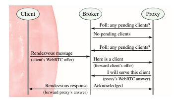
Figure 2: The long-polling communication model of Snowflake rendezvous. Proxies poll periodically to check for new clients. When the broker makes a match, the proxy gets the client's SDP offer, then immediately re-connects to send back its SDP answer. It all happens during one round trip from the client's perspective. Not shown here is the indirect channel used by the client to access the broker through the censor's zone of control (shaded background).
